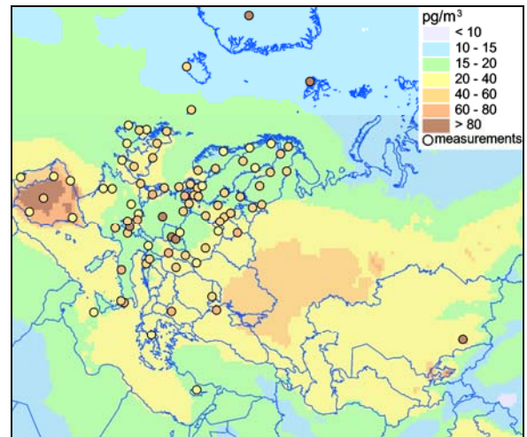
Fig. 3.22. Spatial distribution of modelled HCB concentrations in air obtained for 2006 and measurement data of passive sampling campaign of EMEP carried out in 2006, \text{pg}/\text{m}^3
